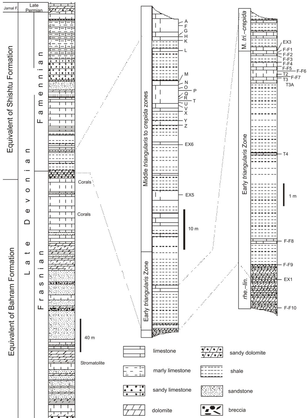
Fig. 5. Stratigraphic column of the Chahriseh section, the column has been closed up two times to show detailed lithology and sampling
